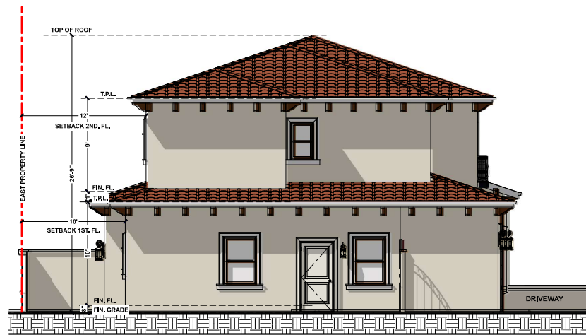
TYP. NORTH ELEVATION, UNITS 1,2,3
