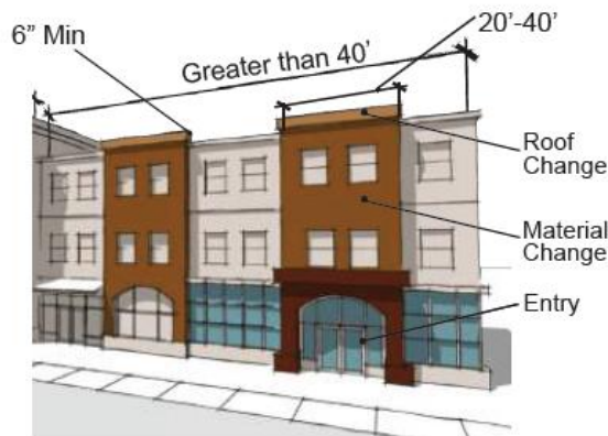
Figure 17.134-11: Building Facade Form Variation
